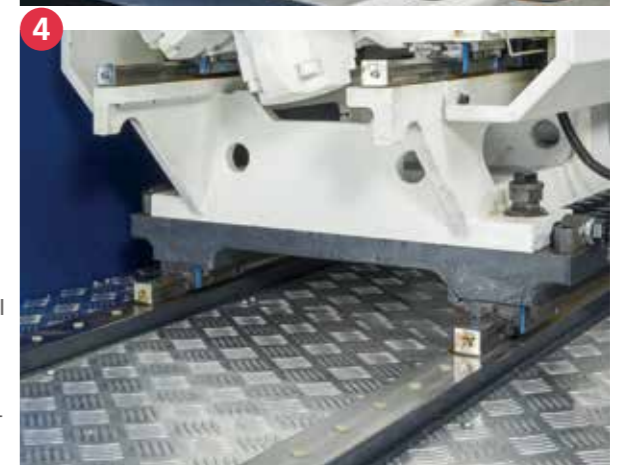
Figure④ Stable high-speed injection through dynamic balanced twin-cylinder, and linear guide rail support improves accuracy.
