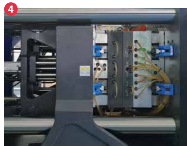
Figure ① The customized special steel tie bar and reinforced safety design meet the requirements for fast cycle times and long life.
